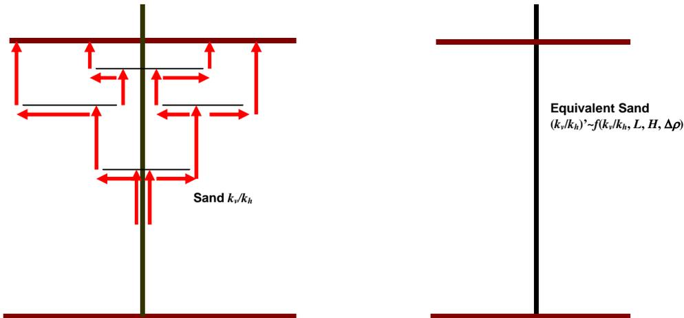
**Figure 3:** Plume direction in reservoir with imbedded shale barriers and its equivalent homogeneous model
