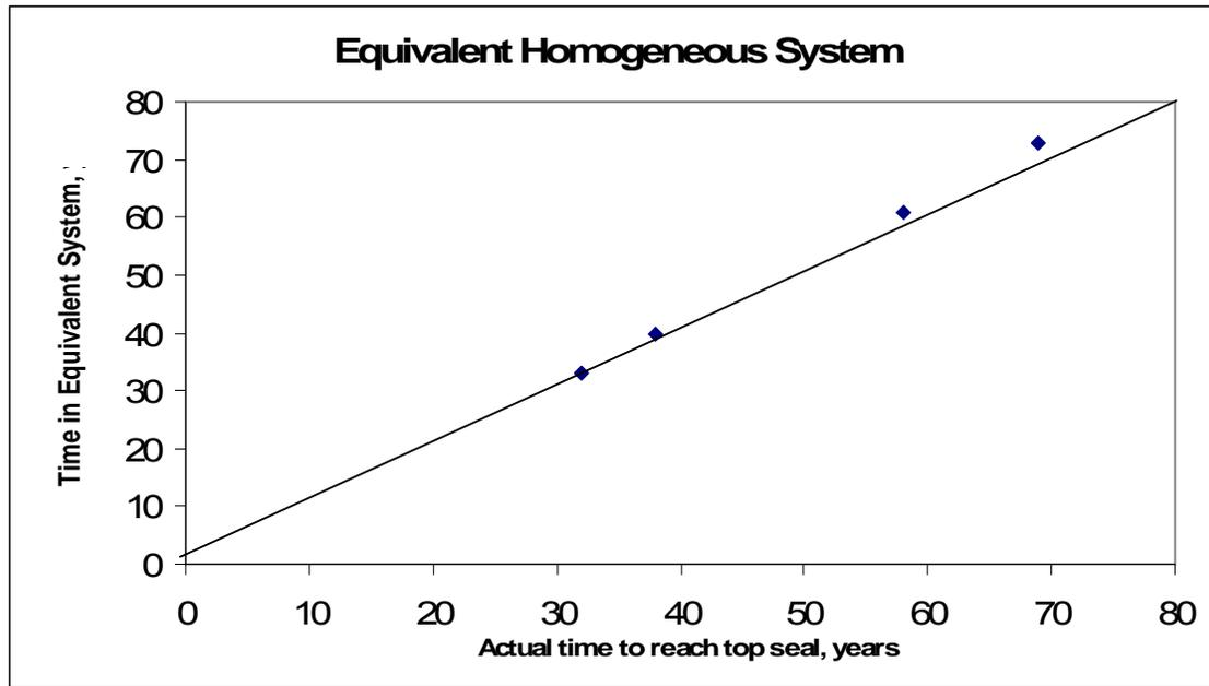
**Figure 4:** Time taken by plume to reach the top seal in shale imbedded aquifer and respective equivalent homogeneous system. The equivalent system allows quick, inexpensive estimation of this response variable.
