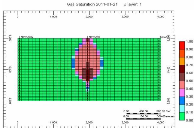
**Figure 5:** CO<sub>2</sub> distribution along the well length at three different times
