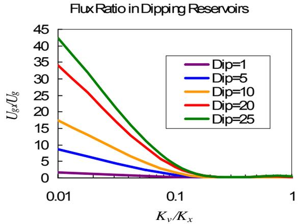
**Figure 2:** Flux ratio as a function of permeability ratio and dip angle
