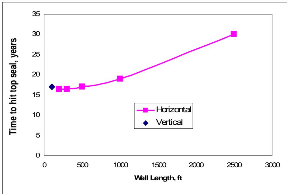
**Figure 7:** Effect of horizontal well length on time to hit top seal.
