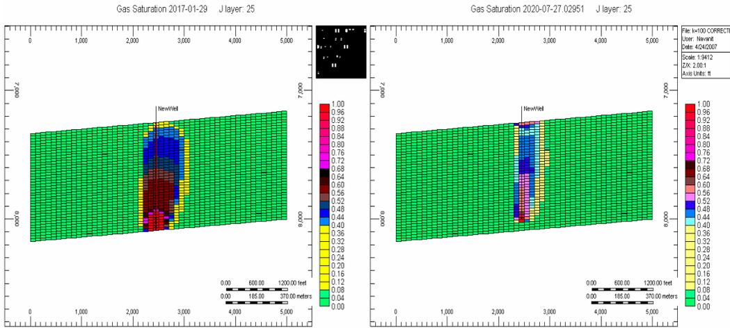
**Figure 6:** CO<sub>2</sub> plume shape in aquifer with (left) Vertical well (right) Horizontal well. Vertical well shows more horizontal spread compared to horizontal well. Horizontal well in figure is perpendicular to paper.
