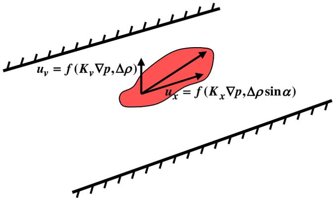
**Figure 1:** Schematic showing plume behavior in dipping reservoir
