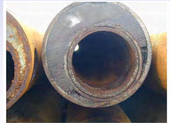
Figure 5-5: Close up of 7 and 10 3/4-in. Casing on the Rack
