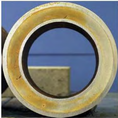
Fig. 10—Conventional cement after cycling.
